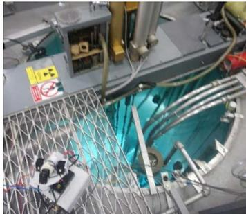
Fig. 17. Stand-off radiation imaging on the reactor platform showing the instrument developed in this research and the reactor pool.
