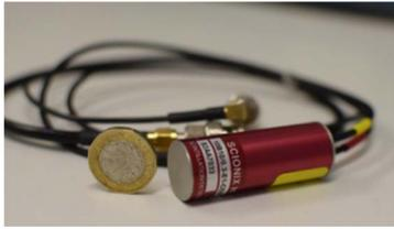
Fig. 2. The CeBr<sub>3</sub> detector used for this research with a UK \$1 coin to indicate scale.
