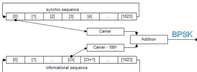
Fig.5– Modulation scheme
