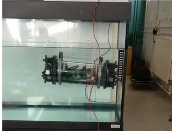
Figure A.3: Snapshot of AVEXIS<sup>TM</sup> from video showing its depth hold capabilities (video available at <https://youtu.be/bEK0zR1iH-E>)
