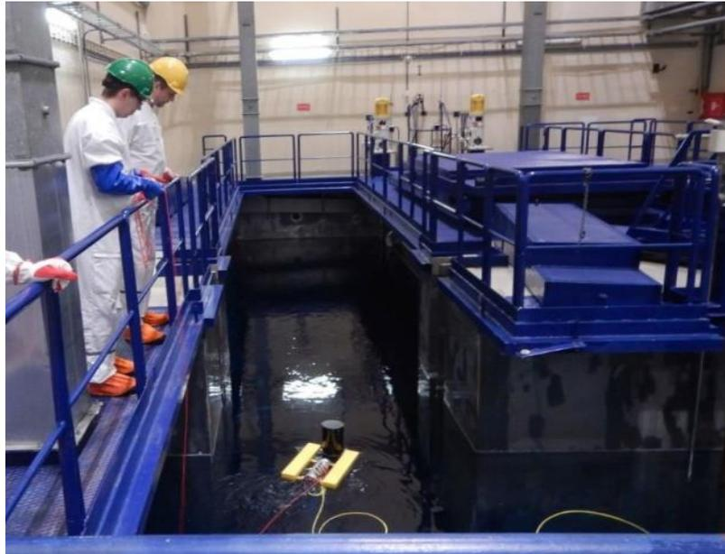
Figure 2 USV KAERI deployed at an interim spent fuel storage pond.
