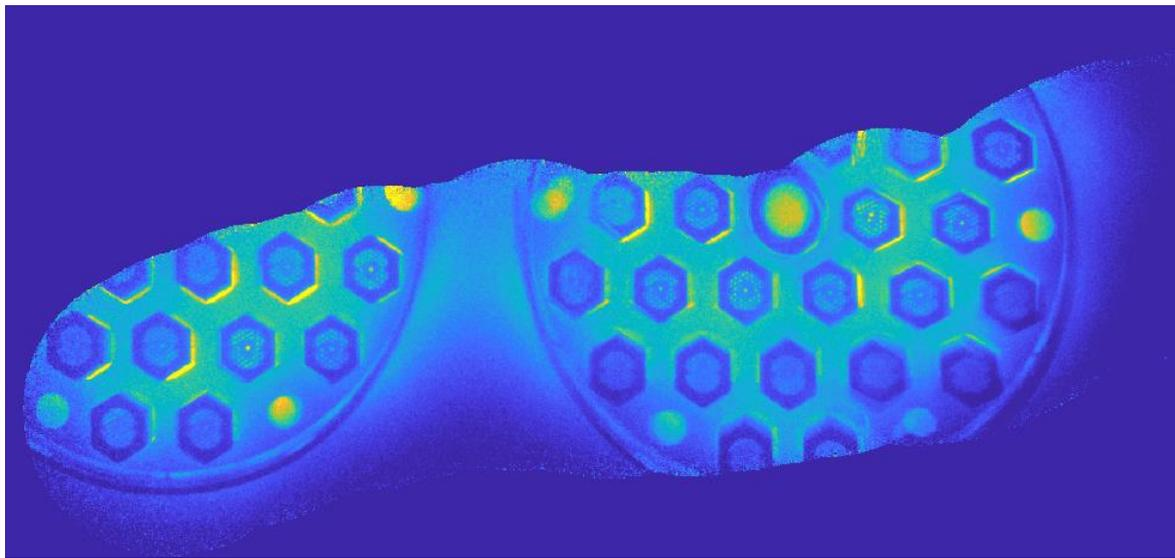
Figure 6 Assembly map built through USV: current XCVD algorithm does not deal well with the rotations of the USV (artifacts visible at the edge of the circles); the slight balancing of the USV when swimming against a water pump makes it difficult to work with longer exposure values, desirable for better sensitivity, but an internal gimbal would help.
