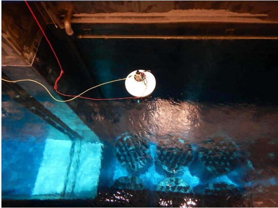
**Figure 3** USV Datastart deployed at an interim spent fuel storage pond. Note the strong surface turbulences, generated by the water pumps that could not be turned off for safety reasons, preventing any potential ICVD verification from the surface.
