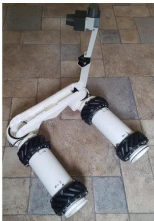
Figure 4. MIRRAX in its driving and sensing configuration. When in a cell the wheel segments fold to make a stable platform and the sensor package is raised.
