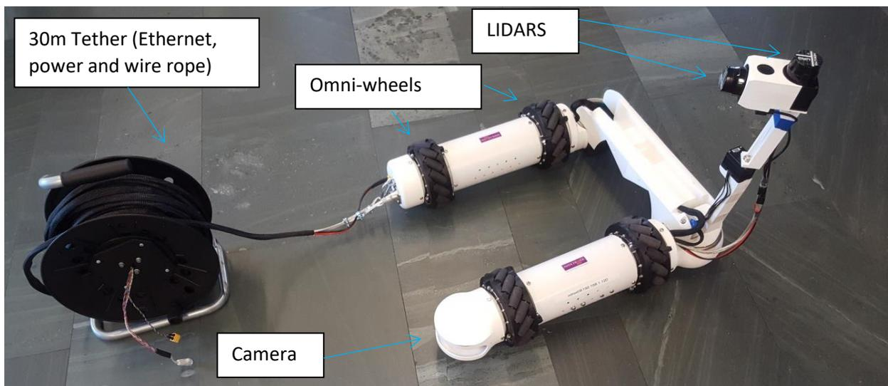
Figure 7. Current prototype of MIRRAX that will be deployed on Sellafield
