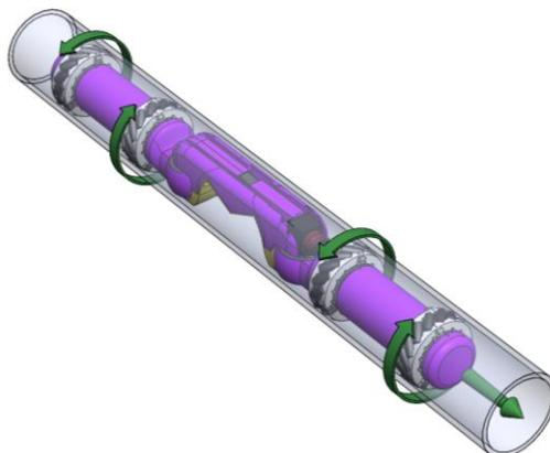
Figure 3. MIRRAX driving through an access port. The omni-wheels alternating directions moves the robot parallel to the wheel axes so it can drive through a tube.
