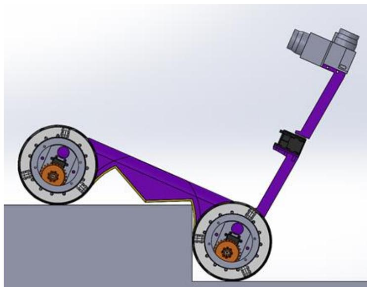
Figure 6. Ground clearance when descending steps. Also shows positions of pinion gear driving wheels (orange)
