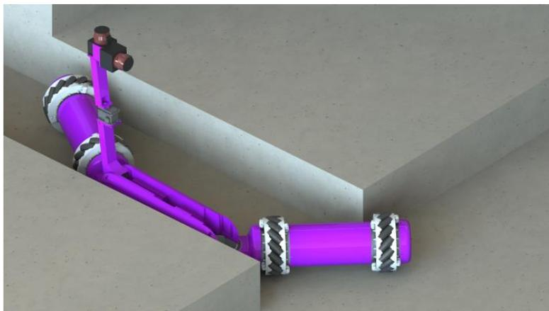
Figure 5. MIRRAX maneuvering obstacles. The wheel segments can be folded into different configurations to maneuver around obstacles while still remaining fully controllable.
